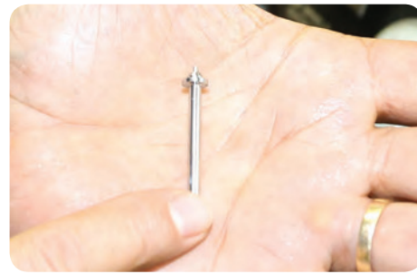
Elmo Vilchez demonstrates pinch turning which is using two turrets with opposing force to turn close diameters on one of four 6-axis mill turn centers.
