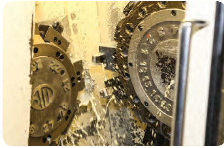
Elmo Vilchez demonstrates pinch turning which is using two turrets with opposing force to turn close diameters on one of four 6-axis mill turn centers.
