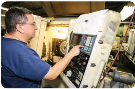
Elmo Vilchez demonstrates pinch turning which is using two turrets with opposing force to turn close diameters on one of four 6-axis mill turn centers.
