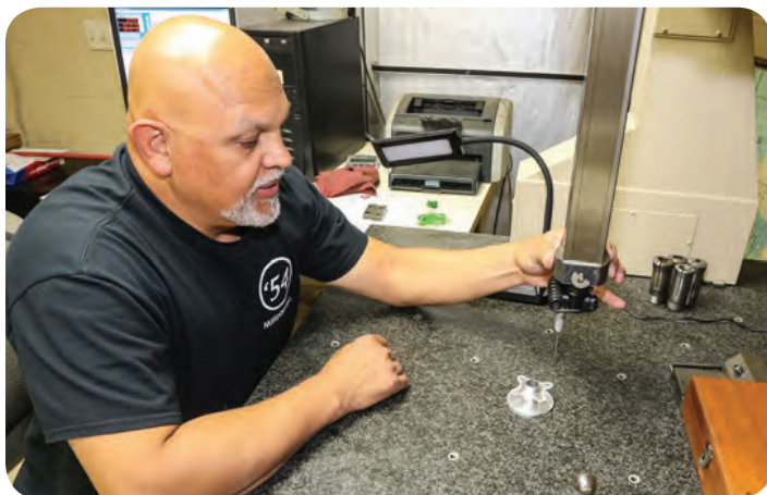
Left - Millipart is ISO 9001: 2008 and AS9100 C Certified. Tom Valles checks parts on the Mitutoyo brand CMM. Right - Millipart specializes in commercial and military aerospace parts. Parts range in size and material.
