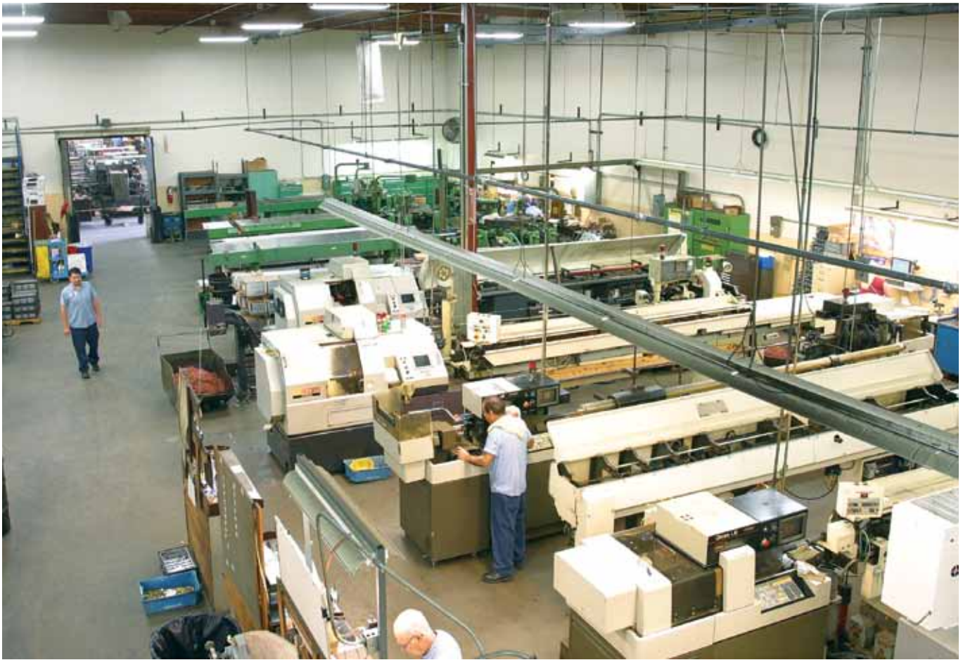
Overview of part of Metric Machining's 45,000-sq-ft facility. The company has 94 employees and runs multi-spindle New Britain screw machines, Davenport's, single-spindle Brown & Sharpe's, Hydromats, CNC lathes and mills, cam and CNC Swiss-style screw machines, and centerless grinders. The 38-year-old company produces parts for some of the biggest names in the aerospace, agriculture, electronics, automotive and offroad vehicle industries.
