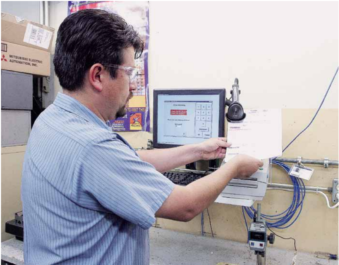
CNC leadman Rafael Quiroz uses a bar code scanner linked to a live Weiss terminal, which, in turn is linked to the company's central server. Data goes into and comes from Visual EstiTrack which automatically tracks job costs, machining time, etc. The operators need only to enter the number of parts made, which significantly improves accuracy of job cost reports.
